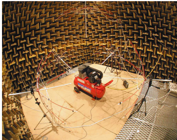
Fig. 10. The air compressor and five microphone arrays in the anechoic chamber.
